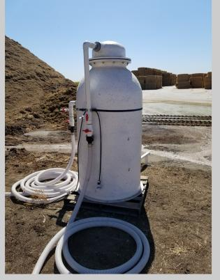
An example of an HPPG-10 Pilot used on a dairy farm in Merced, CA This pilot was used to take influent and effluent samples in order to showcase the filter's effectiveness at removing solids from the water post-screen.
